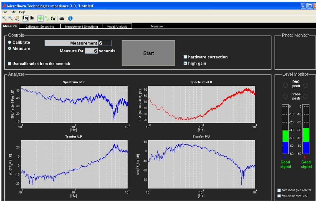
**Figure 5: Spectrum of P, Spectrum of U, Transfer U/P and Transfer P/U in Rigid Pavement**
