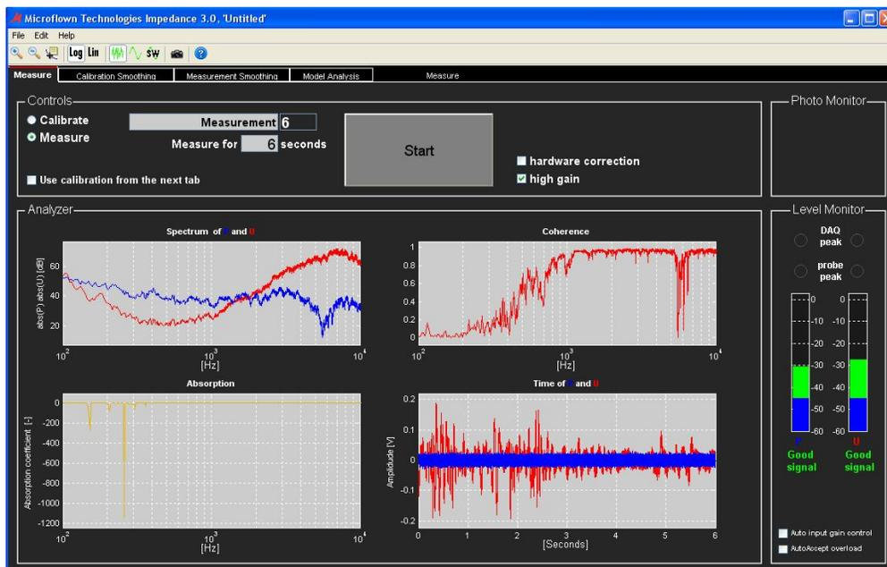
**Figure 3: Spectrum of P&U, Coherence, Absorption and Time of P&U in rigid pavement surface**
