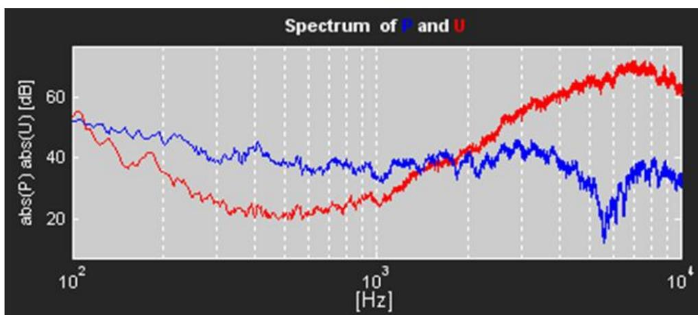
**Figure 9: Spectrum of P & U in Rigid Pavement**
