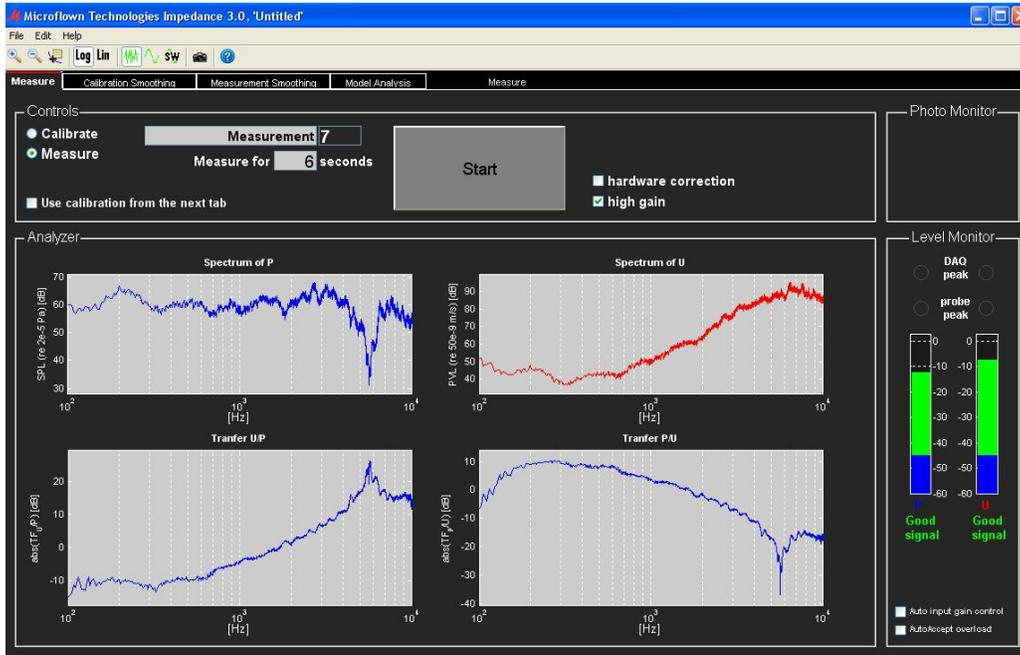
**Figure 6: Spectrum of P, Spectrum of U, Tranfer U/P and Tranfer P/U in Flexible Pavement**
