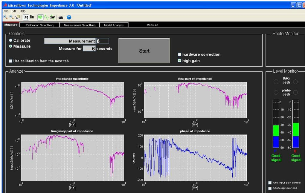
**Figure 7: Impedance magnitude, Real part of Impedance, Imaginary part of Impedance and Phase of Impedance in Rigid Pavement**
