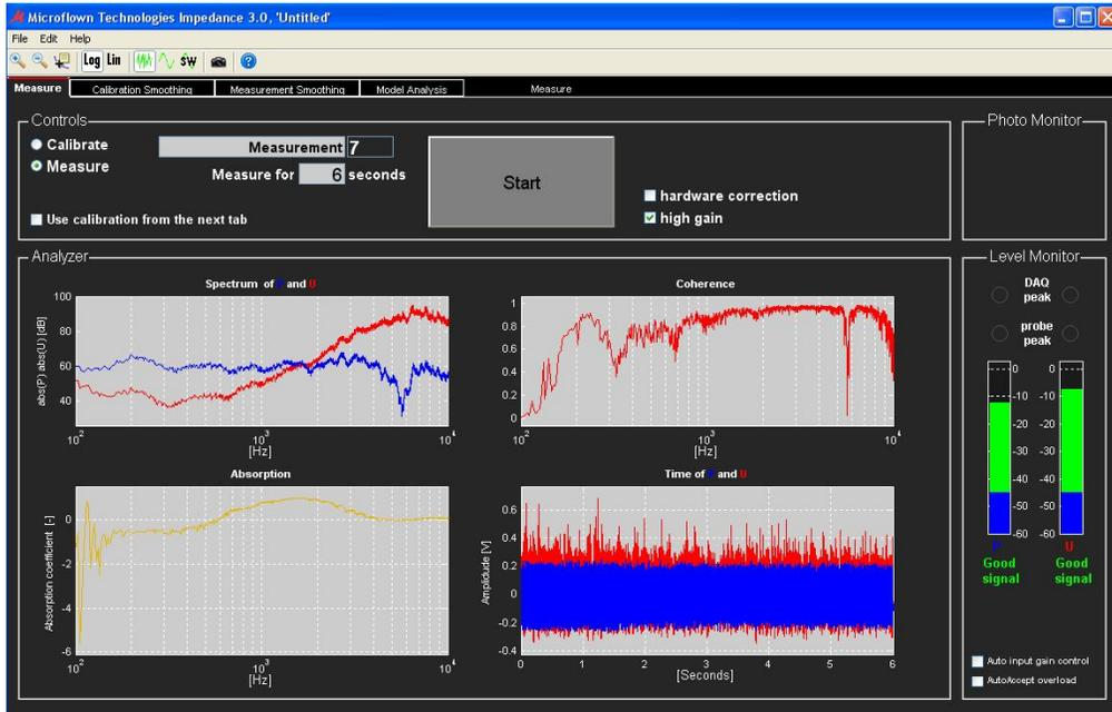
**Figure 4: Spectrum of P&U, Coherence, Absorption and Time of P&U in flexible pavement**
