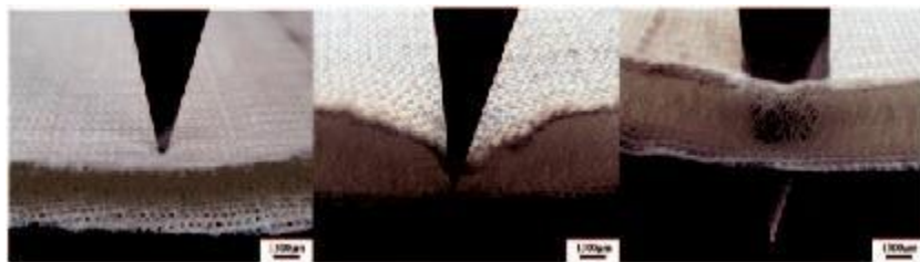
Figure 2: The Puncturing Process of Warp-Knitted Spacer Fabric
