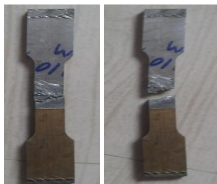
Figure 3: Tensile Test Specimen before and after Test
