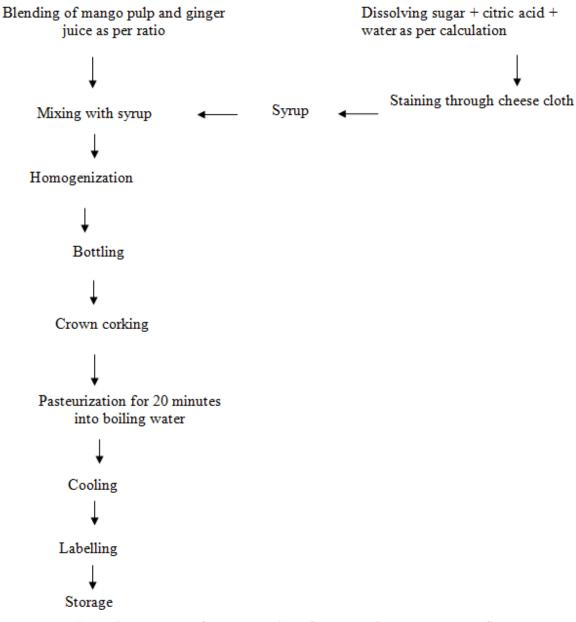
Figure 3: Flow sheet for preparation of mango- ginger blended RTS
