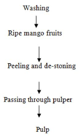
Figure 1: Flow sheet for extraction of pulp from ripe mango fruits
