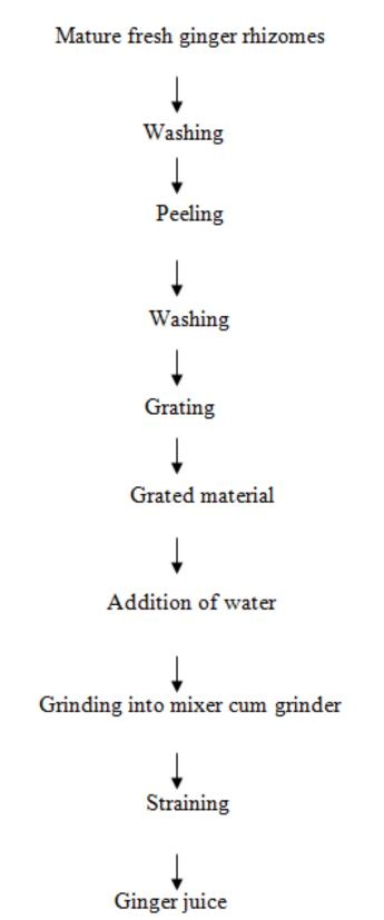
Figure 2: Flow sheet for extraction of juice from fresh ginger rhizomes
