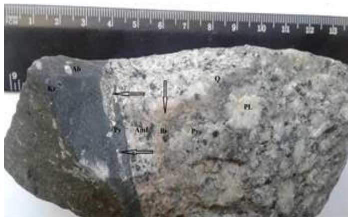
Figure 3: Contact of the granodiorite of the Koytash intrusion with the dike of the andesibasalt (sample UP-8) with pronounced kalifeldsparization with impregnation of pyrite (the arrow indicates the zone of kalifeldsparization and sulphidization, the symbols denote the name of the minerals)
