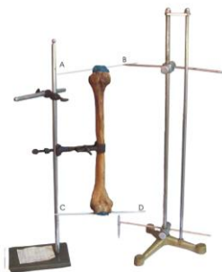
Fig. showing Parallelograph and osteophore with a fixed humerus bone. AB and CD are the axis of the two ends demarcated by pins fixed with plasticin.
