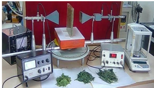
Figure 1: X- band Microwave Set-up for measuring Attenuation due to Tree Leaves by Free Space Method
