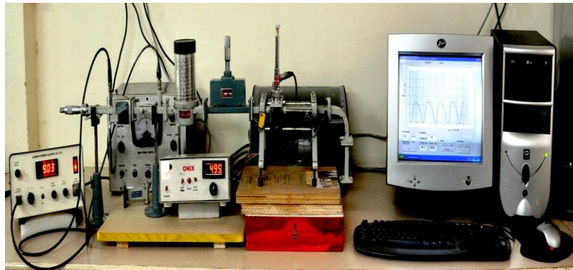
Figure 2: X- band Microwave Set-up for measuring Dielectric constant of Tree Leaves by Waveguide cell Method
