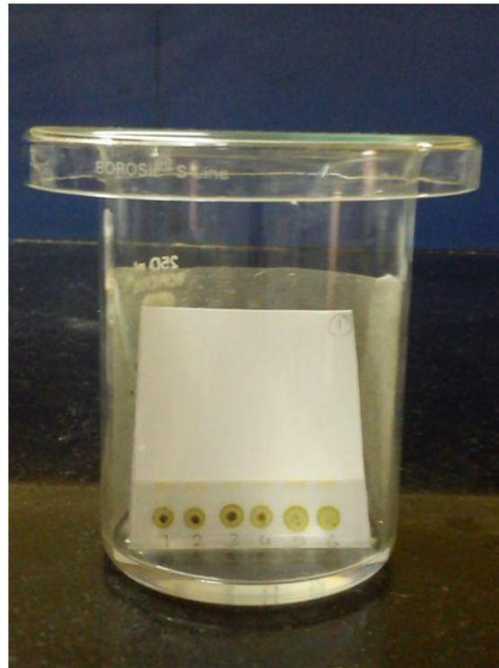
**Figure 2: Developed in benzene as solvent**
