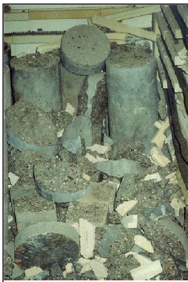
Figure 1 Explosive spalling of HPC when heated to 700 0 C (Sideries et al. 2009)
