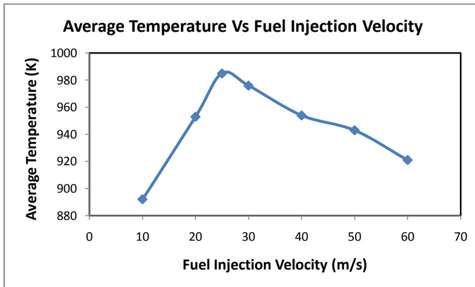
**Figure 3: Variation of average temperature with fuel injection velocity**
