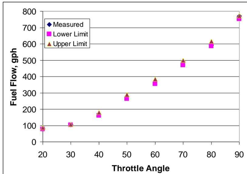
**Figure 9: Throttle Valve Calibrations**
