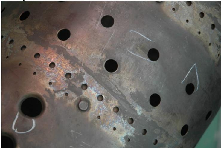
**Figure 5: Combustor Flame Tube Cracks**
