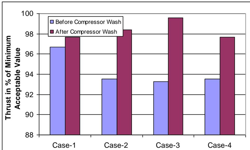
Figure 2 Thrust of the sampled engines
