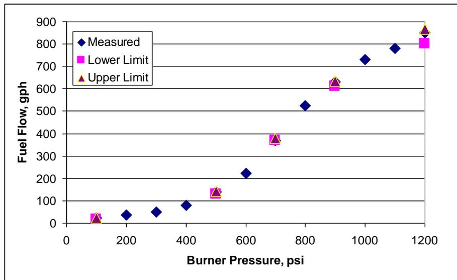
Figure 10: Atomizer Calibration
