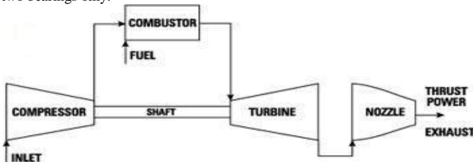
**Figure 1: Schematic Layout of Gas Turbine engine**
