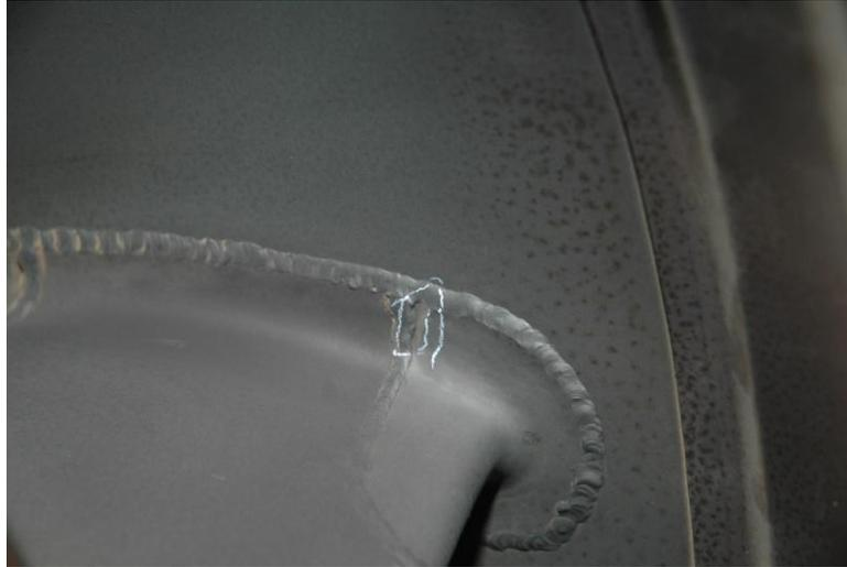
**Figure 8: Cracks in Exhaust Cone**
