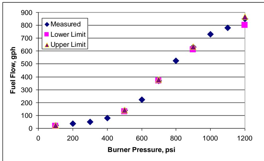
Figure 10: Atomizer Calibration
