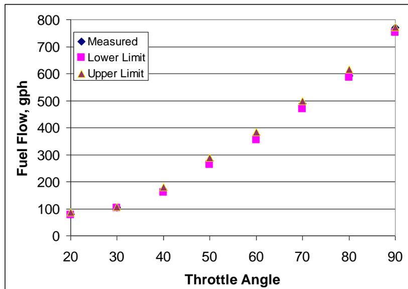
**Figure 9: Throttle Valve Calibrations**
