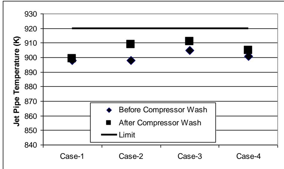
**Figure 3: Jet Pipe Temperatures of the sampled engines**
