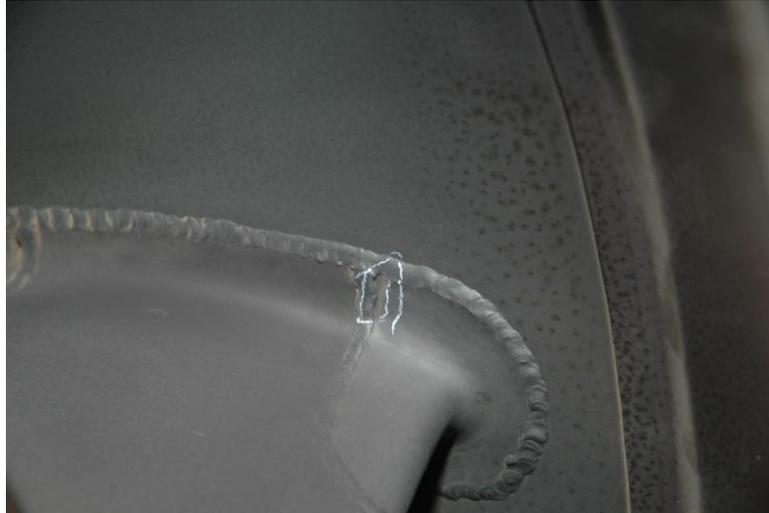
**Figure 8: Cracks in Exhaust Cone**
