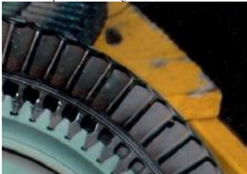
Figure 7: Condition of Turbine Assembly after completion of one TBO Life
