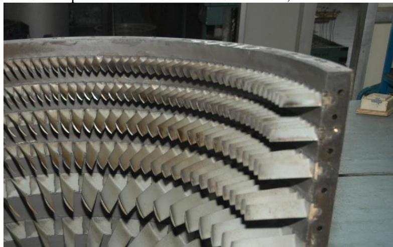
Figure 4: Compressor Casing and Stator vane assembly
