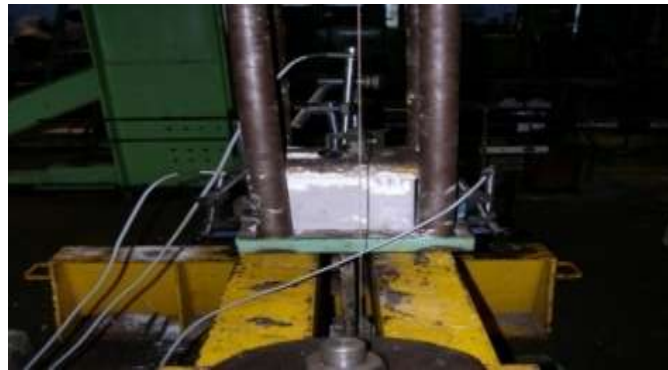
Figure 2: Test set-up and arrangement of LVDTs
