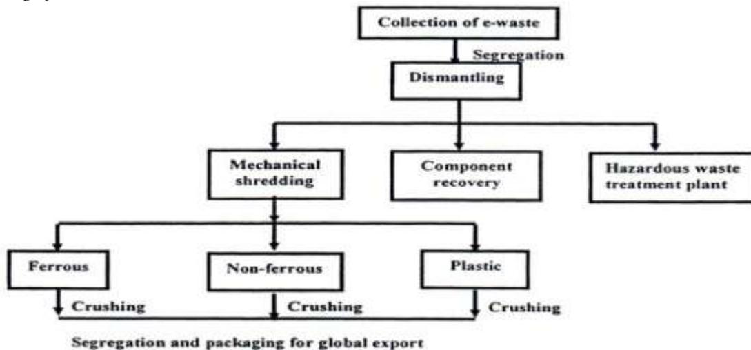
**Figure 2: Schematic flow diagram for the recycling of w-wastes in Indian Industry Jha *et al.*, (2011)**
