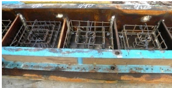
Figure 3: Casting of anchorage Specimen,
