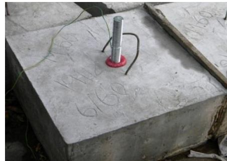
Figure 4: Fabricated Anchorage Specimens.
