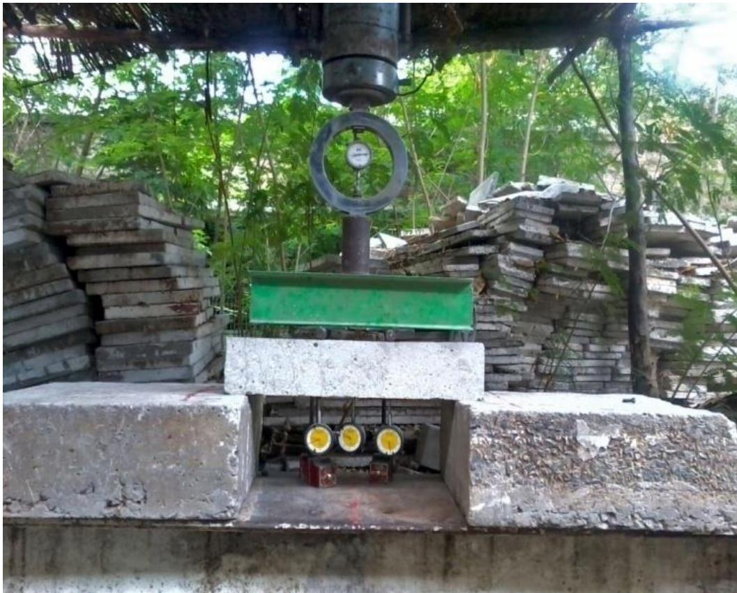
Figure 2: Testing of Beam for Flexure
