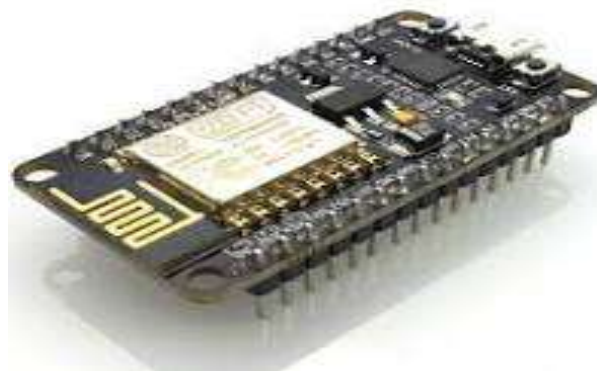
Figure 1: Node –MCU is a module based on ESP8266 Wifi module. USB TTL included ,plug and play module.
