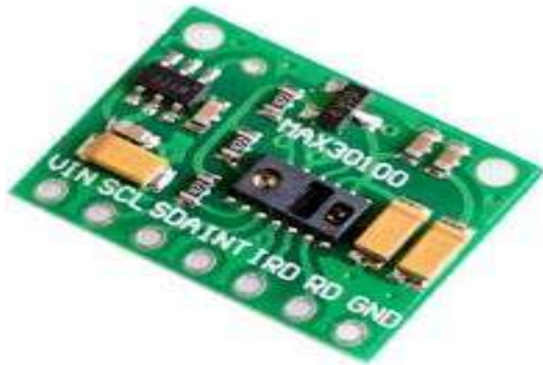
Figure 3: MAX 30100 is an integrated pulse oximeter and herat rate monitor sensor solution . Input voltage 1.8v to 5.5v.
