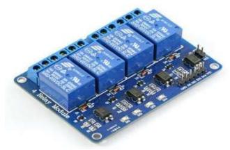
This is a 5V 4-channel relay interface board, and each channel needs a 15-20mA driver current. It can be used to control various appliance and equipment with large current. It is equipped with high-current relays
