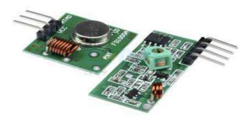
The RF module comprises of an RF transmitter and an RF receiver. The transmitter/receiver (Tx/Rx) pair operates at a frequency of 434MHz. An RF transmitter receives serial data and transmits it wirelessly through RF through its antenna connected at pin4. The transmission occurs at the rate of 1Kbps – 10Kbps. The transmitted data is received by a receiver operating at the same frequency as that of the transmitter.
