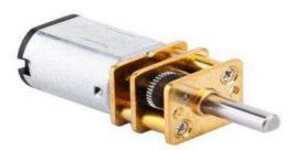
The 30 Rpm Gear Motor and 500 Rpm Gear Motor are used to move forward, reverse and cleaning the waste which is present inside the sewage pipe.
