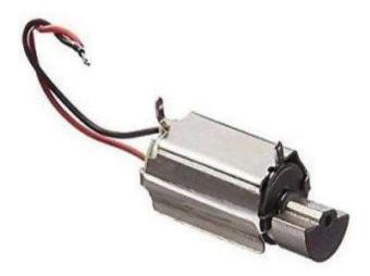
The cylindrical shape is also called bar-type vibration motor. This vibrating motor is essentially a motor that is improperly balanced. In other words, there is an off-centered weight attached to the motors rotational shaft that produces a centrifugal force while rotating. This unbalanced force displaces the motor. Moreover, increasing the voltage supplied to the motor will increase its speed, and therefore the vibration frequency, as well as the vibration amplitude
