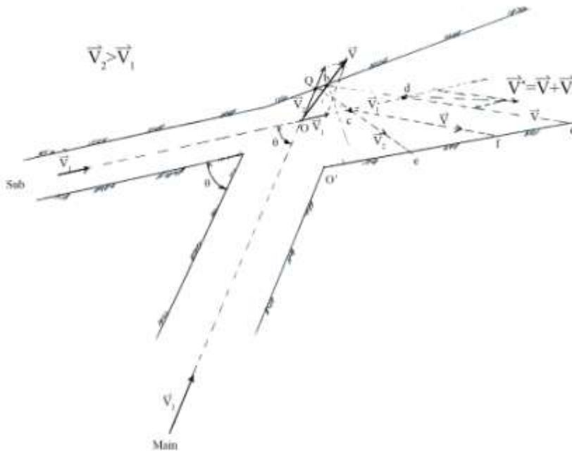
**Figure 2: (2) Confluence Flow: the stronger velocity in main-channel**
