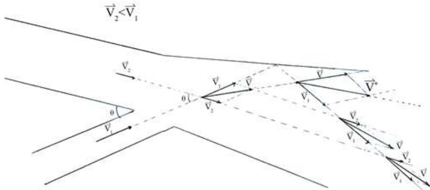
**Figure 3(2): Confluence Flow: the stronger velocity in sub-channel**
