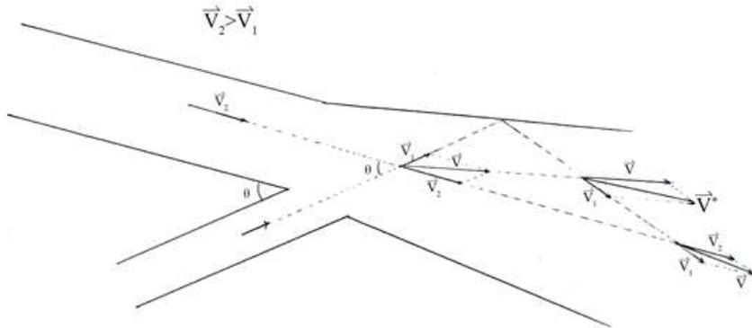
**Figure 3 (1): Confluence Flow: the stronger velocity in main-channel**
