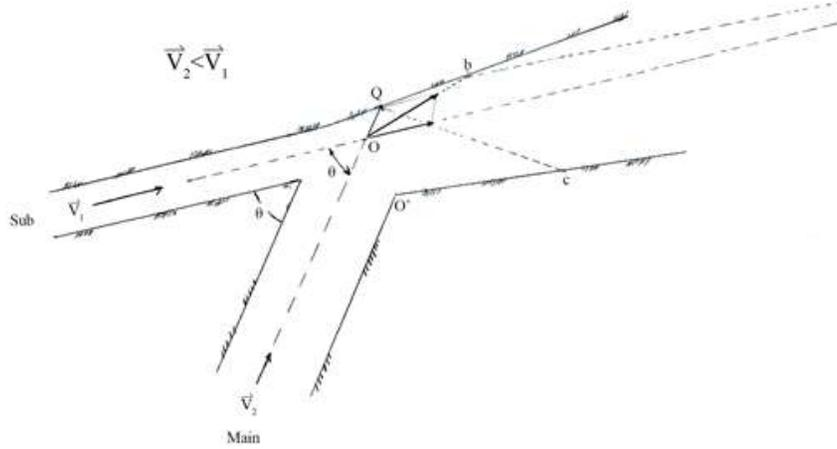
**Figure 2: (1) Confluence Flow: the stronger velocity in sub-channel**
