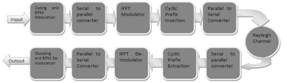
OFDM is simply defined as a form of multi-carrier modulation where the carrier spacing is carefully
