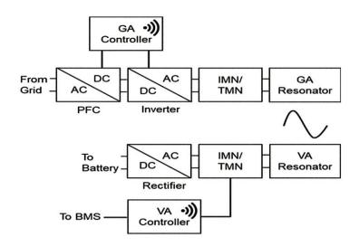
Block diagram of EVs wireless Charging, Where VA is vehicle assembly and GA is ground assembly.
