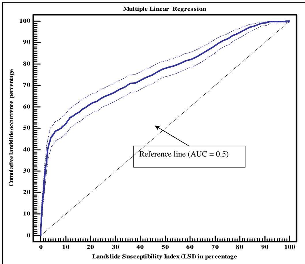
**Figure 12: Cumulative frequency diagram showing success rate curve for susceptibility maps produced by Multiple Linear Regression model hazard map**
