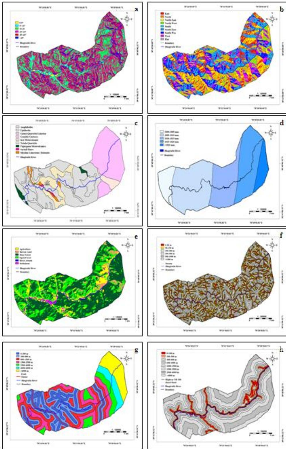
**Figure 7: Input thematic layers of Uttarkashi area: (a) Slope gradient map, (b) Slope aspect map, (c) Lithology map, (d) Rainfall map, (e) Land cover map, (f) Distance from river map, (g) Distance from fault map, (h) Distance from road map**
