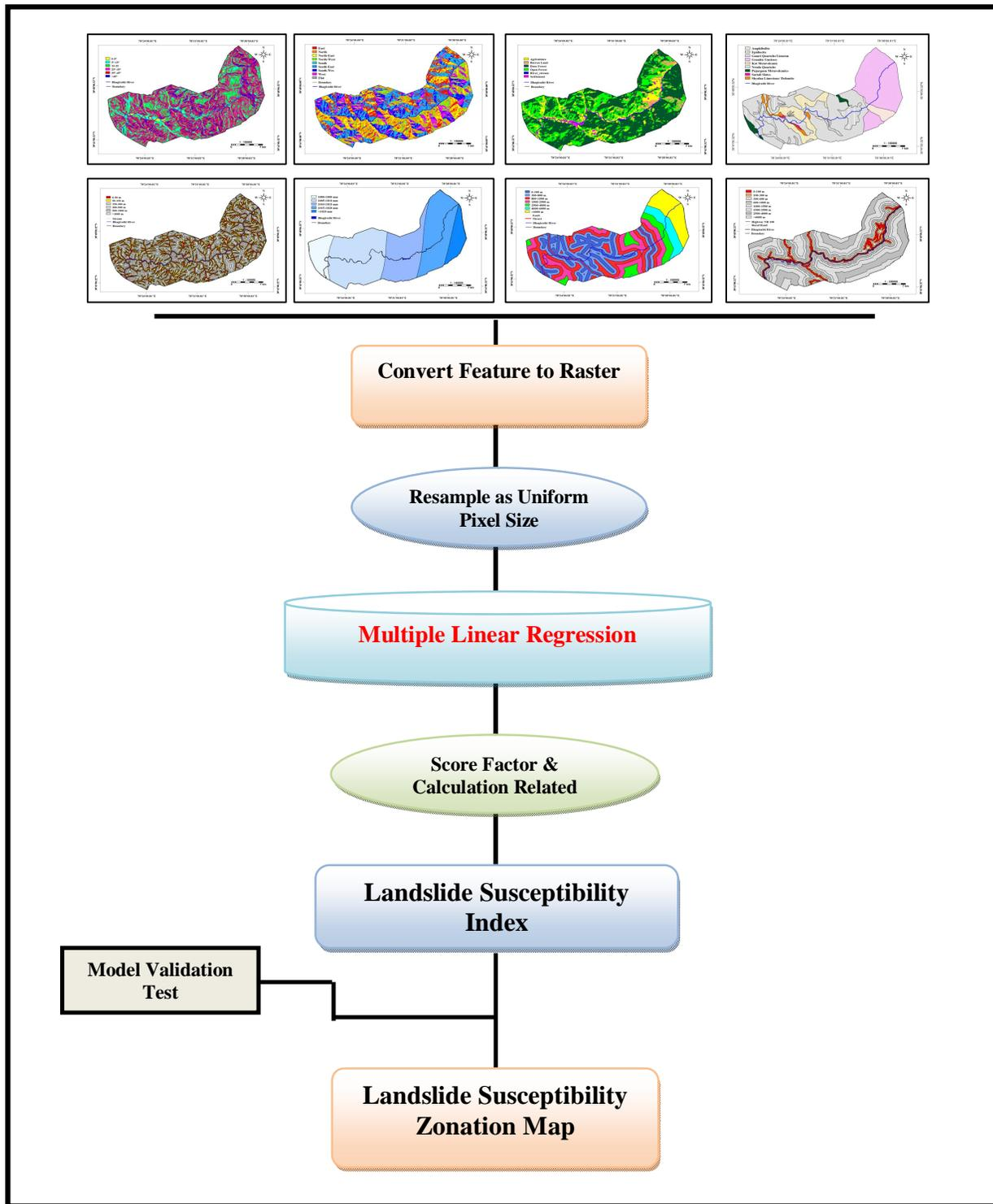
Figure 8: Schematic representation of preparation of LSZ map in Multiple Linear Regression model
