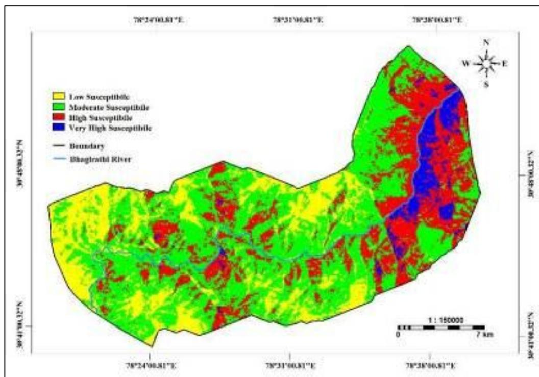
**Figure11: Landslide susceptibility Zonation (LSZ) map**
