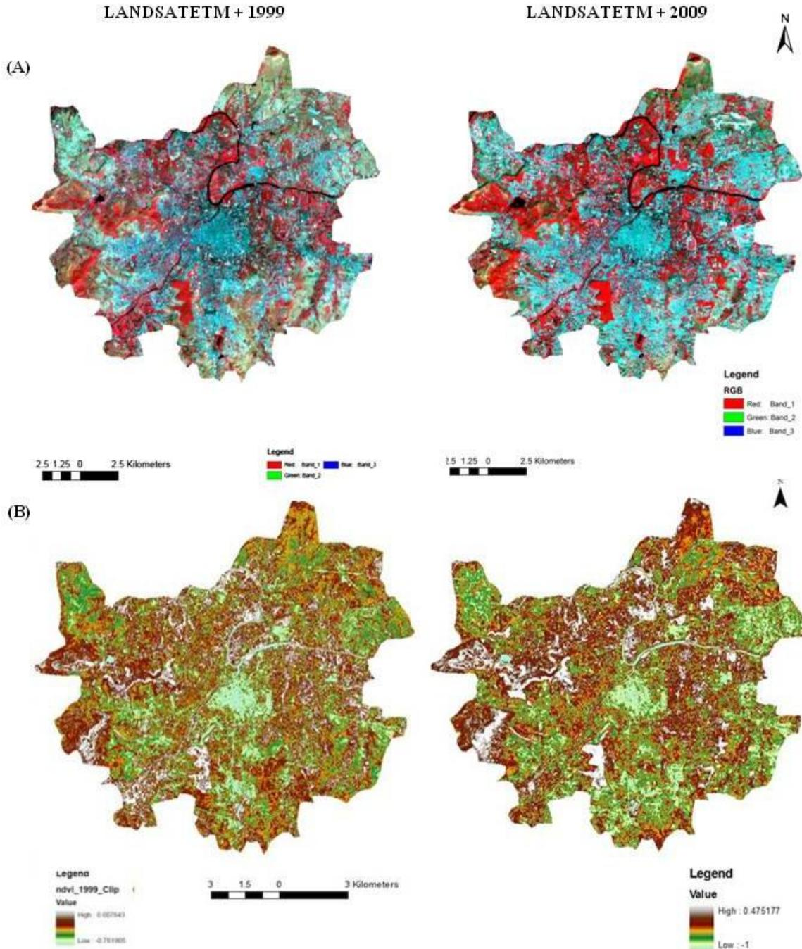
(A) False colour composite images Landsat 7 ETM+ (B) NDVI mapping of Pune city
