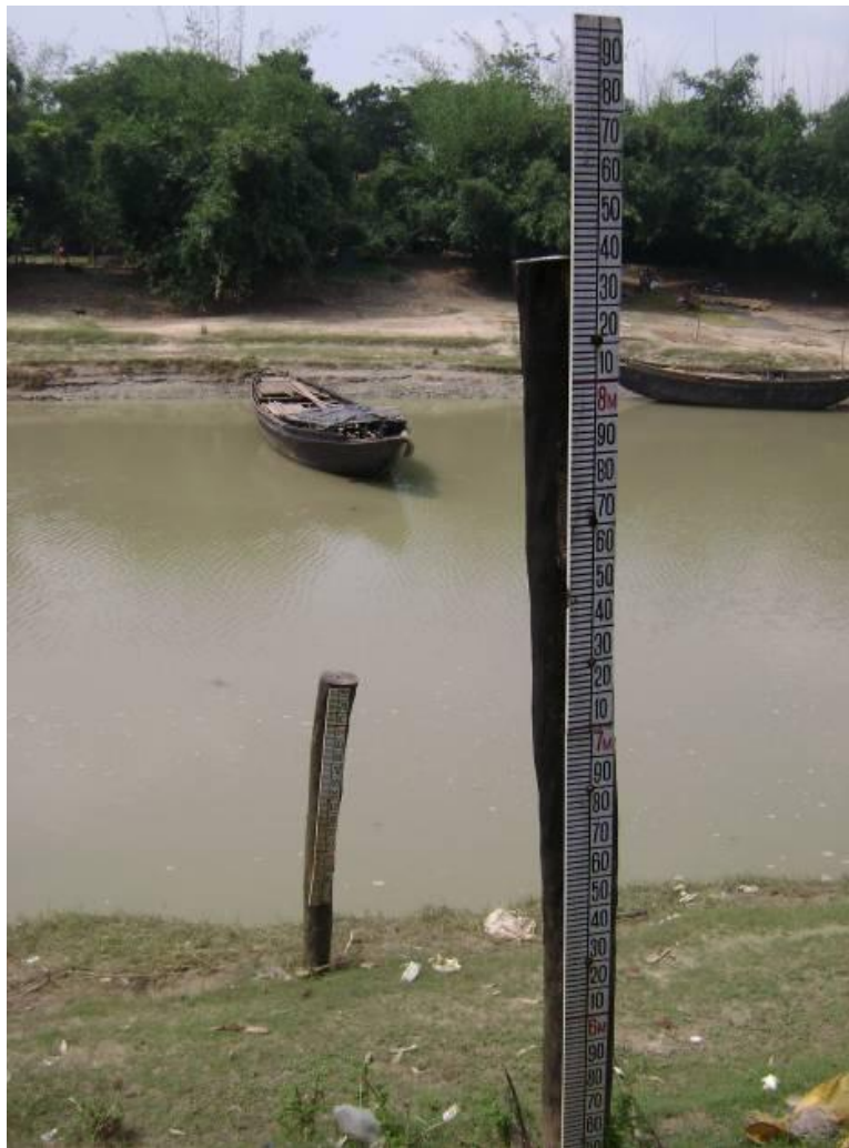
Figure 2: Bank top height measurement at Moyna River bank
