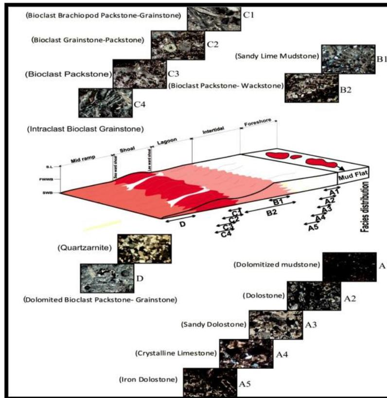
**Figure 2: Three – dimensional modeling of sedimentary platform carbonate – Siliciclastic, Bahram Formation suggested Shamsabad section**
