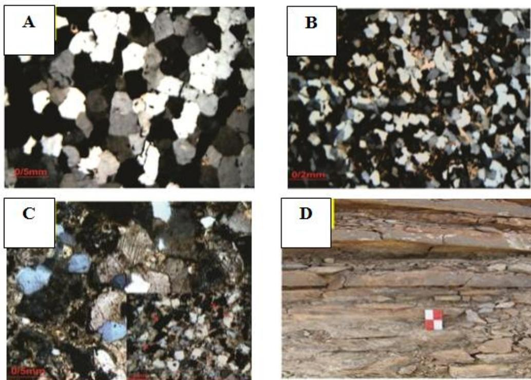
**Figure 5: Photomicrograph of different facies. A: Quartz arenite, XPL. B: Sublitharenite, XPL. C: Calcareous sandstone, XPL. D: Intercalation of Shale and sandstone.**
