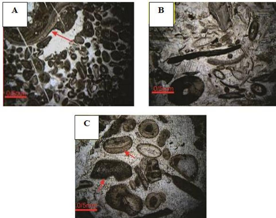
**Figure 9: photomicrograph of barrier. A: Ooid grainstone, PPL. B: Intraclast bioclast grainstone, PPL. C: Ooid bioclast grainstone, PPL.**
