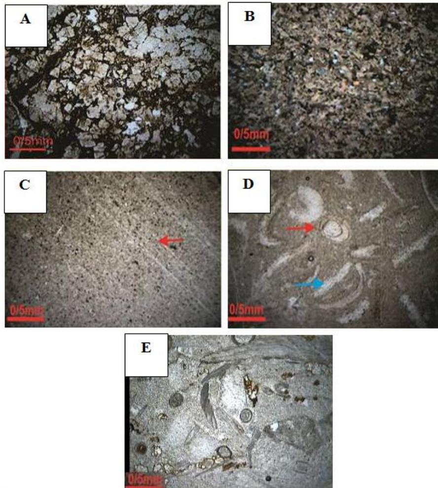
**Figure 6: Photomicrographs of microfacies. A: Dolostone, PPL. B: Dolomitized lime mudstone, XPL. C: Crystalline lime mudstone, PPL. D: Bioclast wackestone, PPL. E: Bioclast intraclast wackestone to packstone, PPL.**
