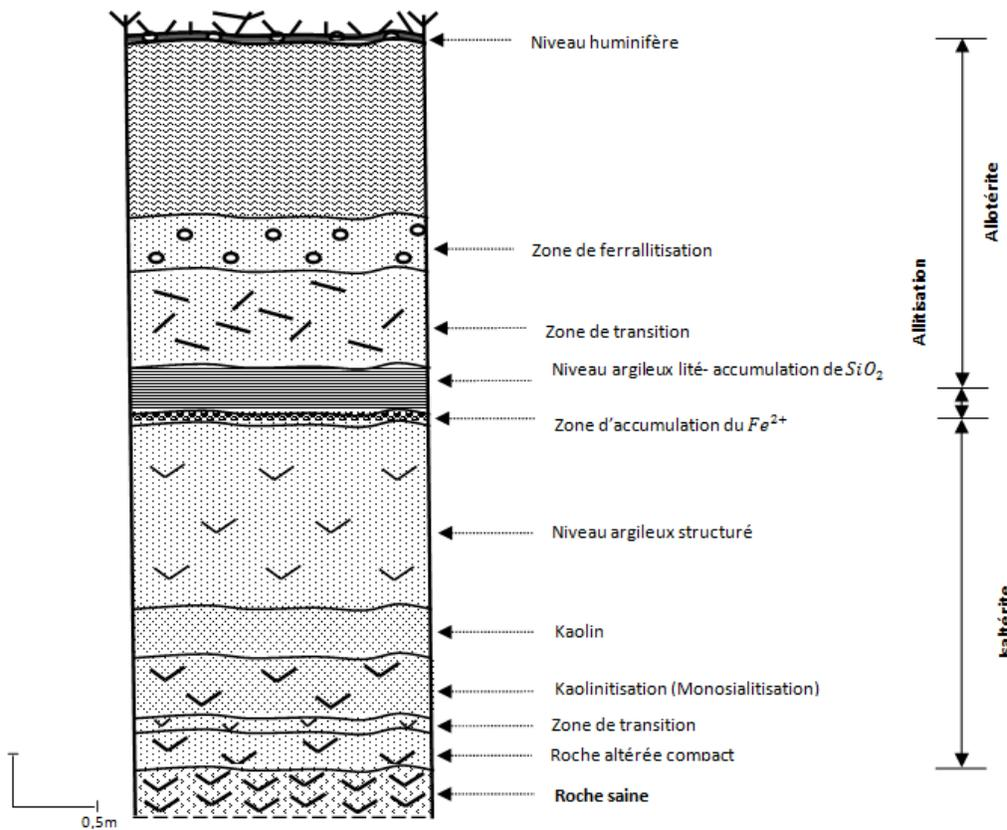
**Figure 1: Weathering profile of Batsingla trchybasalte**
