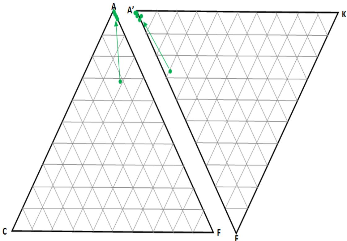
**Figure 8: Oxides A'KF and ACF Diagrams of the batsingla weathering profile showing that the weathering progresses to the "continental" clays**
