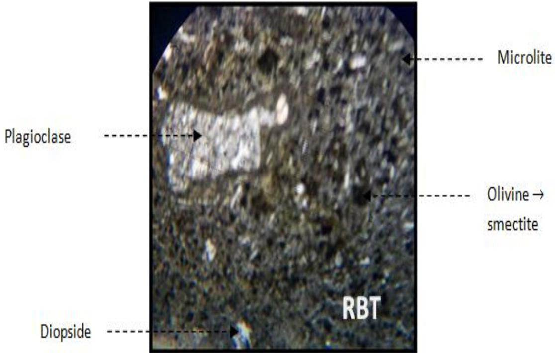
**Figure 7: Image of slightly altered rock in polarized and analyzed light**
