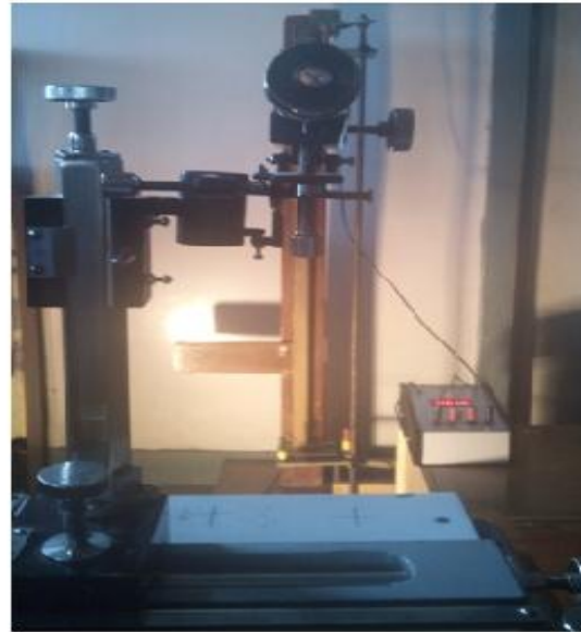
Figure 2: Experimental Set-up with modified telescope for scale reading
