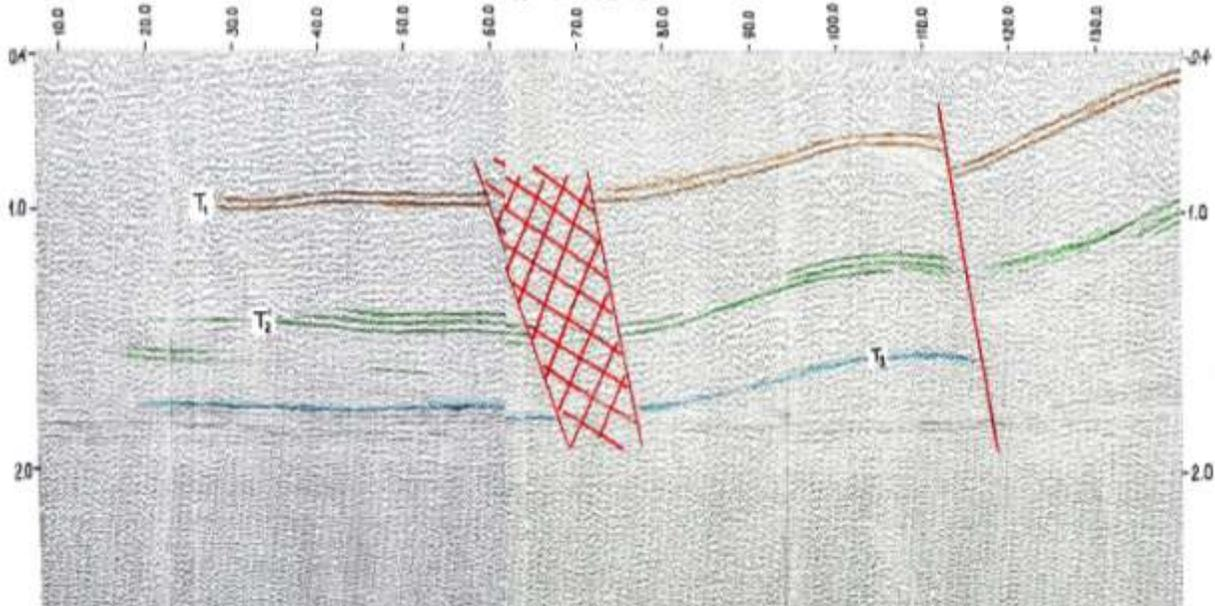
**Figure 3: Time section from 31912491 CDP profile. (Horizontal axis indicates number of pickets and vertical axis is wave travel time, respectively)**
