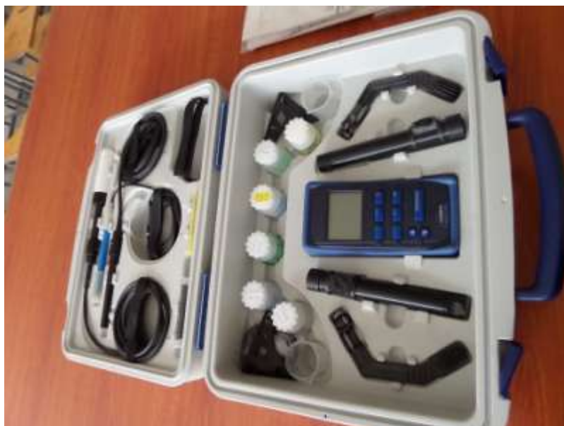
Figure 5: showing the device of pH in the laboratory of Kabul university, Geoscience faculty, department of geology, in this procedure 5g soil (smaller mm sieving passing samples) in the Biker solution and we can find the amount of H + and OH - in the soils.
