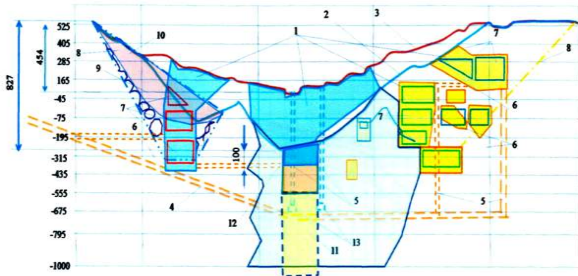
Figure 2: Scheme of the combined development of the deposit when combining open-pit and underground mining operations at the Muruntau deposit
