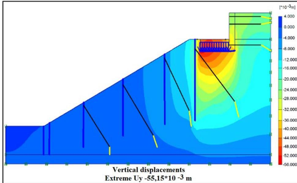
**Figure 20: Settlement after reinforcement by a sheet pile wall system**
