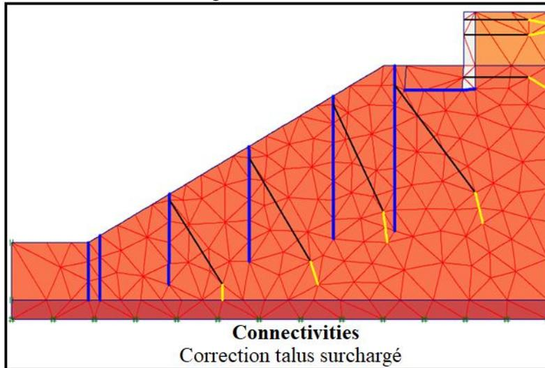
**Figure 16: Mesh of the slope reinforced by a sheet pile wall system**
