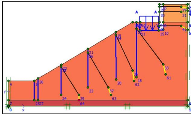
**Figure 15: Slope model reinforced by a sheet pile wall system**
