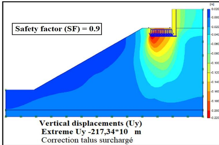
**Figure 8: Settlement due to the abutment load**
