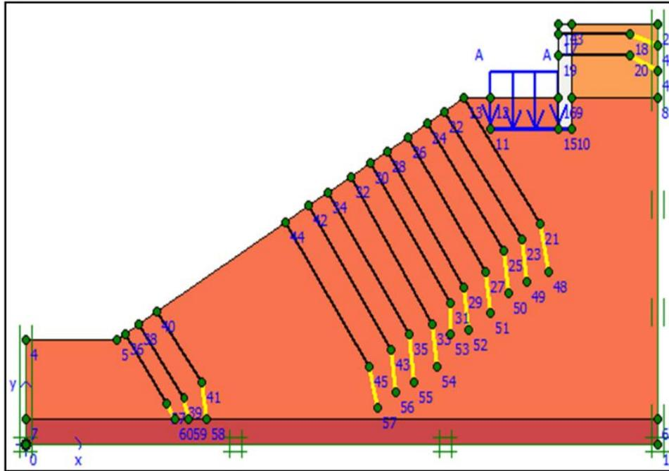
**Figure 9: Slope reinforced model by anchoring associated with geogrids**
