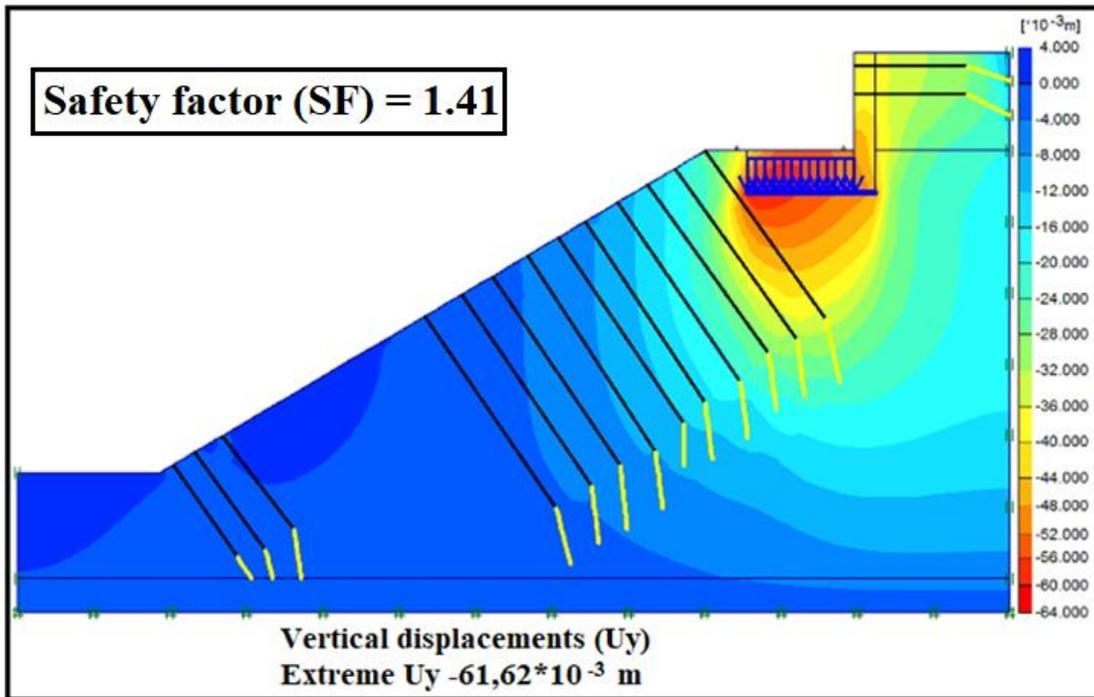
**Figure 14: Settlement after reinforcement by anchoring**
