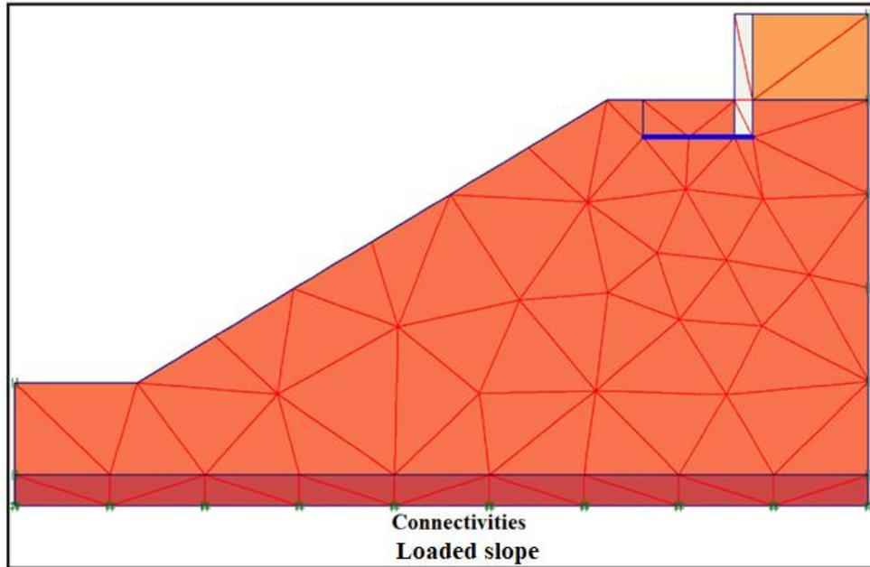
**Figure 4: Mesh of the embankment loaded by the abutment (C3)**
