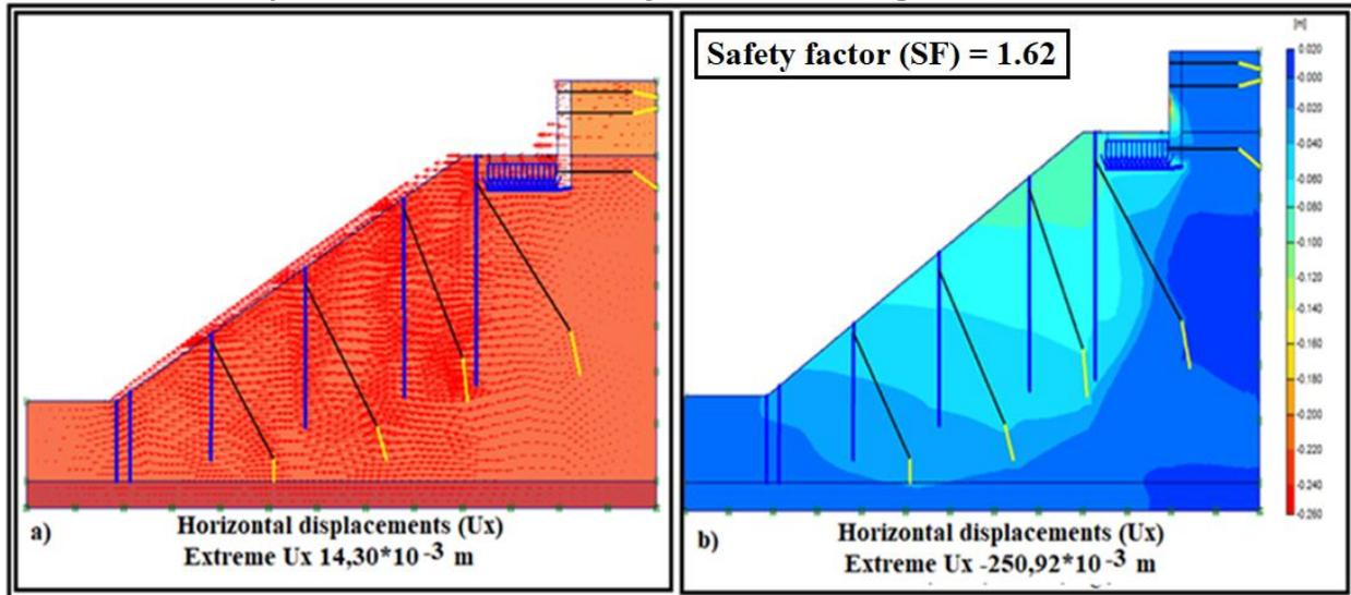
**Figure 19: Horizontal displacement**
