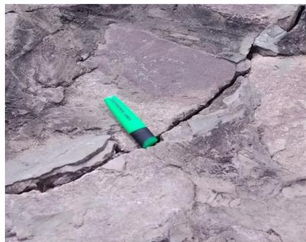
**Figure 2: Photo of the shear plane observed on the slope (fracture)**
