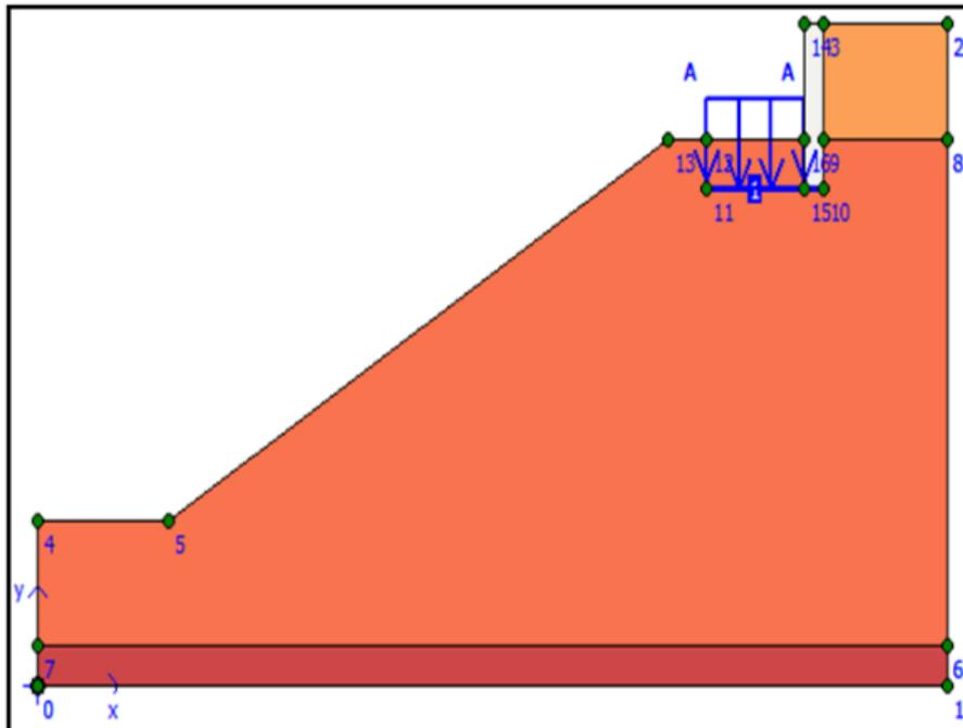
**Figure 3: Geometry model of the loaded slope by Abutment (C3)**
