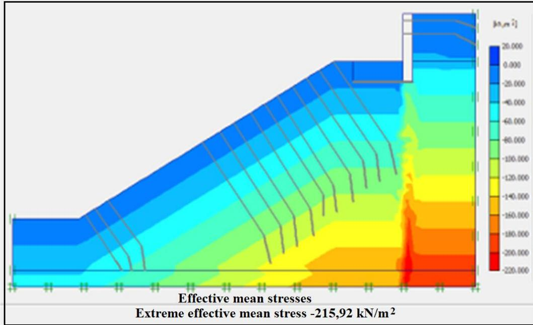
Figure 11: Total initial stresses distribution (-215.92KN / m<sup>2</sup>)
