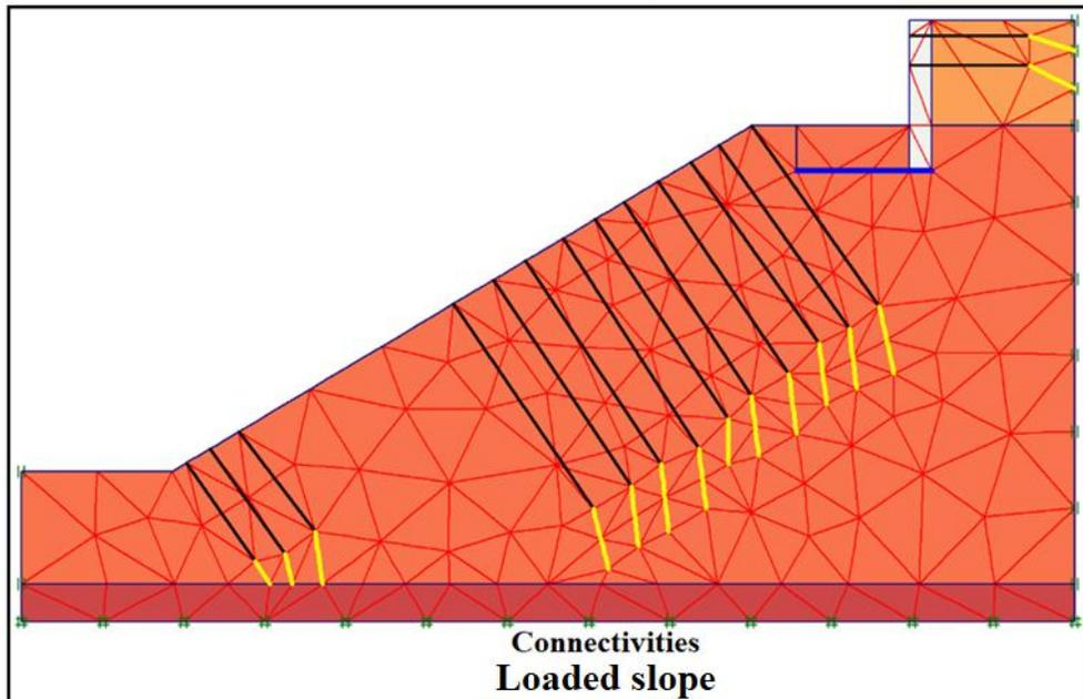
**Figure 10: Slope mesh reinforced by anchoring**
