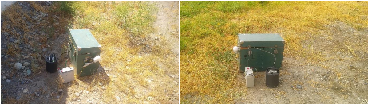
Figure 3: Noise level investigation process using the Guralp 6TD seismometer
