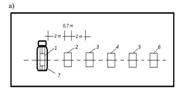
Figure 1. Experimental site at the "Oqtepa" area a) - schematic view. b) - general view. 1-6 - test pits; 7 - vibratory roller.
