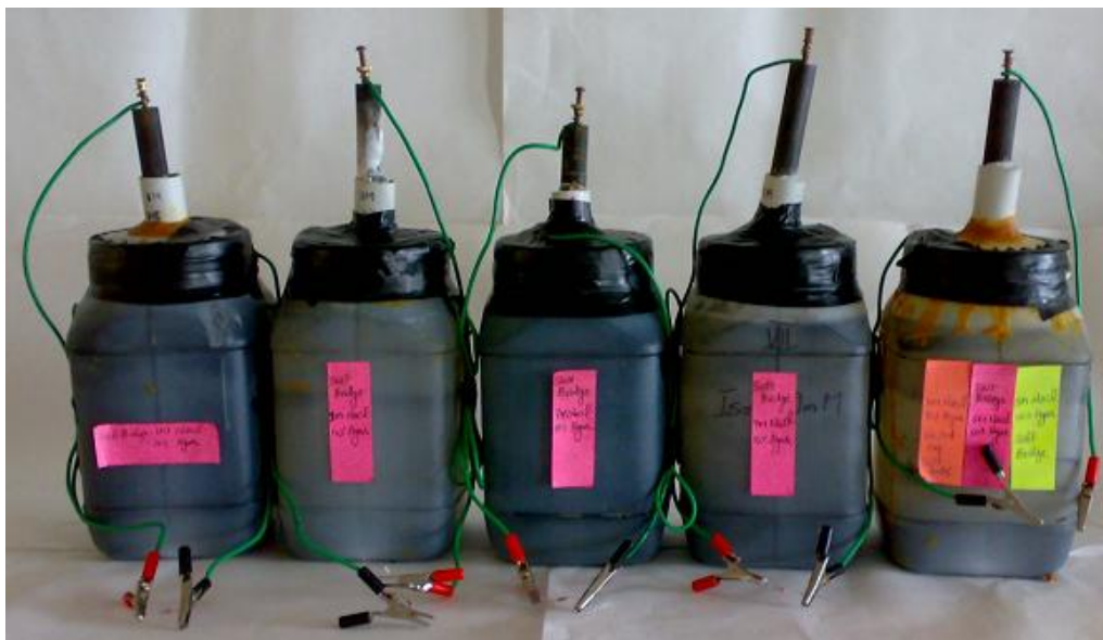
Figure 3. SBIAC MFC with 1, 3, 5, 7, 9M Salt Bridge
