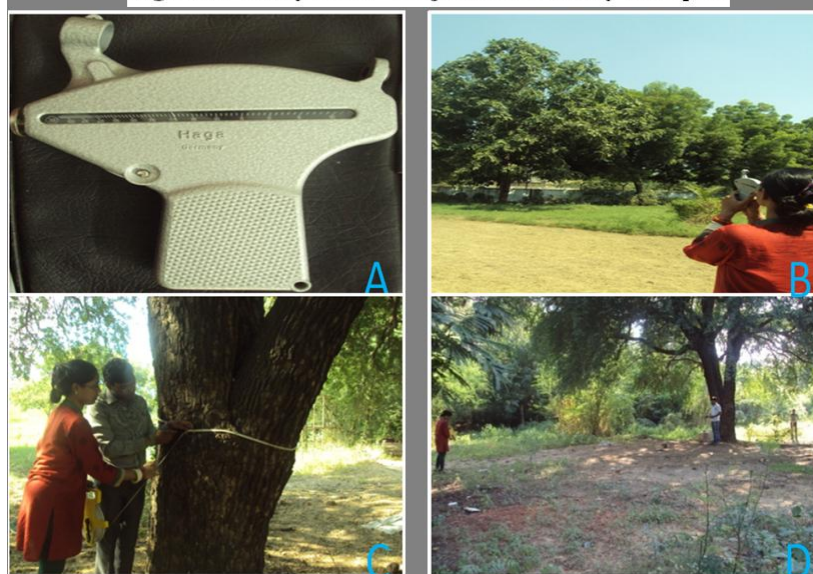
Figure 2: Method of tree biomass computation. A & B: Haga's Altimeter to measure tree height. C: Measurement of GBH. D: Measurement of tree canopy.
