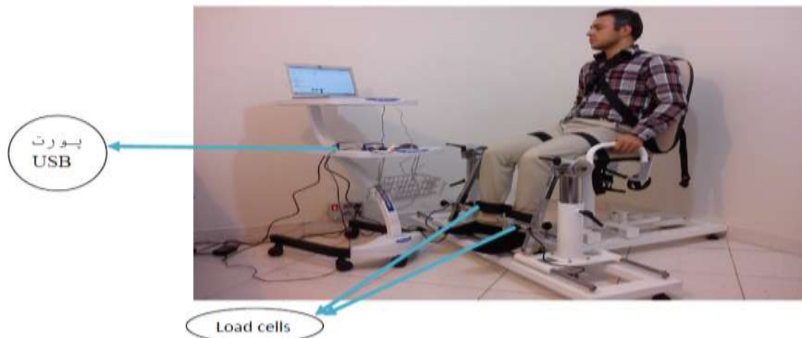
Figure 1: Measurement of Maximal Isometric Contractions and Reproducing the Target Force with the use of Dynamometer
