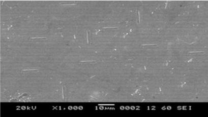
Figure 2: SEM Image of Copper Sulphide Thin Film
