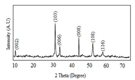
Figure 1: XRD Pattern of Copper Sulphide Thin Film
