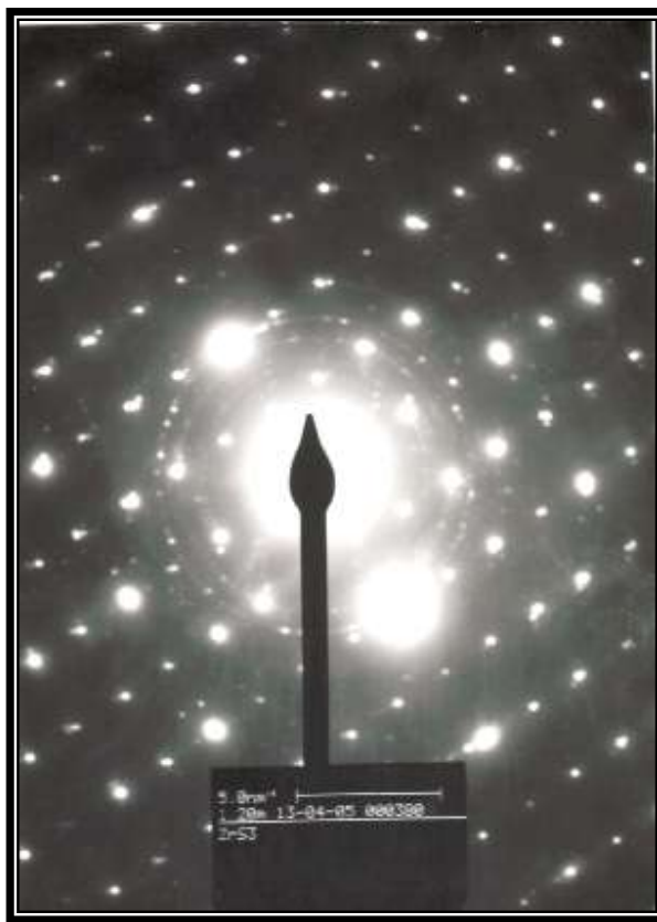
Figure 5: The SAD pattern of as grown ZrS_3 single crystals
