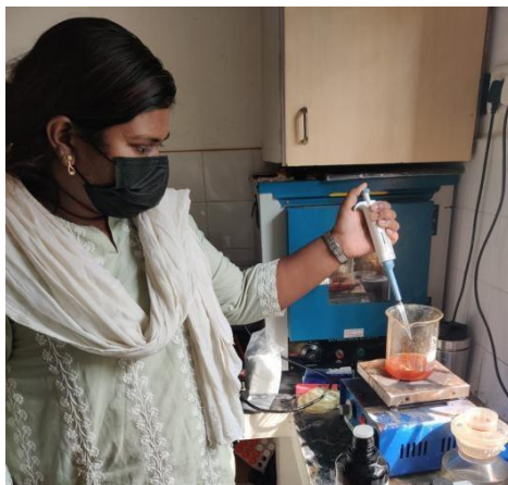
Fig. 2 Magnetic nanoparticles was synthesized using co-precipitation method
