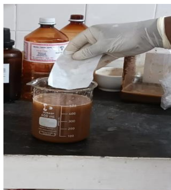
Fig. 7 Spiking of 0.1 ppm of lead acetate
