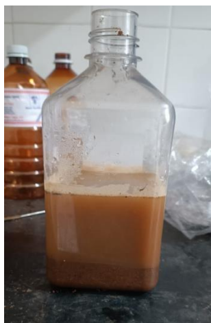
Fig. 6 Soil along with 500 ml of distilled water
