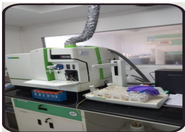
Fig. 8 Inductively coupled plasma optical emission spectrophotometry
