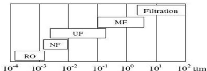
**Figure 2: Basic principles of processes of reverse osmosis, ultrafiltration, microfiltration and filtration**
