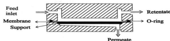
**Figure 4: The cross-section of ultrafiltration cell**
