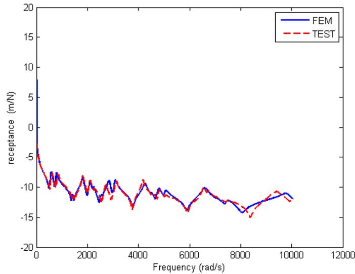
**Figure 1: The comparison of total frequency response functions diagrams of board with a TQFP piece**
