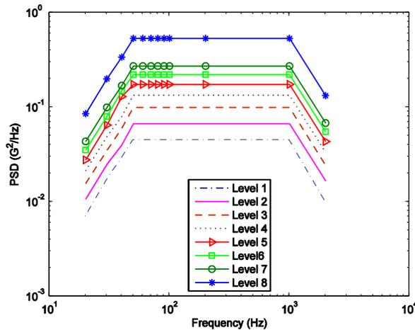
**Figure 2: PSD diagram in 8 input excitation level**
