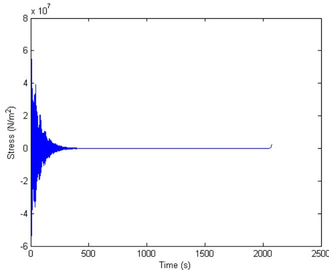
**Figure 3: Stress diagram in time domain for acceleration eighth level**
