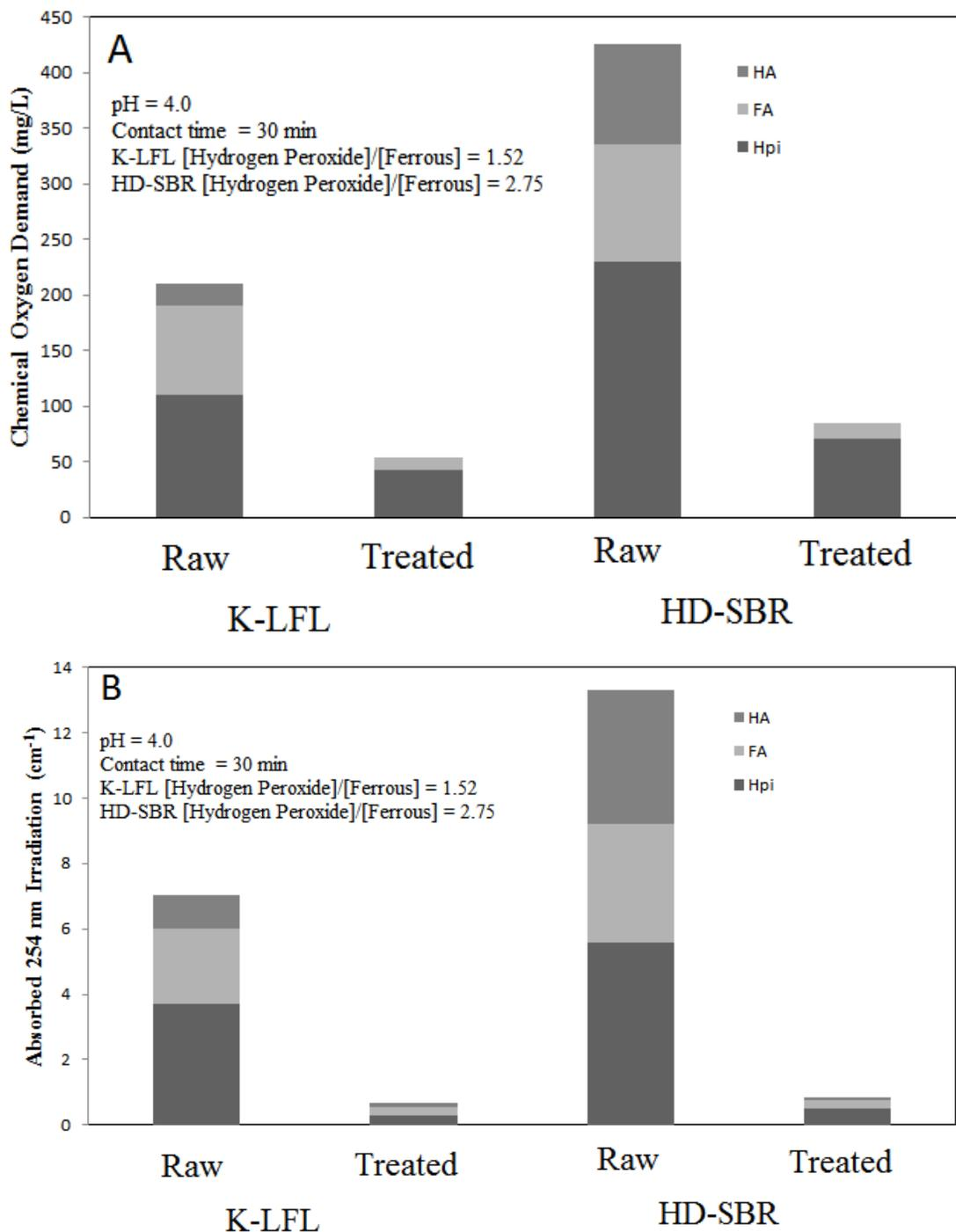
**Figure 3: Distribution of chemical oxygen demand (a) and UV<sub>254</sub> absorbance (b) among the hydrophobic–hydrophilic nature based fractions in the raw and Fenton’s reagent treated K-LFL and HD-SBR landfill leachates under optimized conditions of pH and reagent molar ratio**
