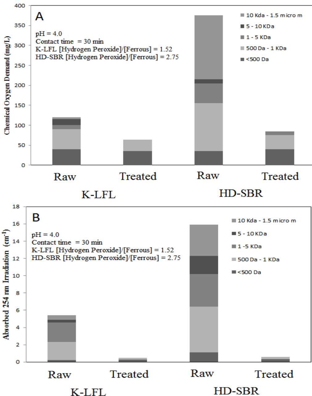
**Figure 2: Molecular weight distribution of chemical oxygen demand (a) and UV<sub>254</sub> absorbance (b) in the raw and Fenton's reagent treated K-LFL and HD-SBR landfill leachates under optimized conditions of pH and reagent molar ratio**
