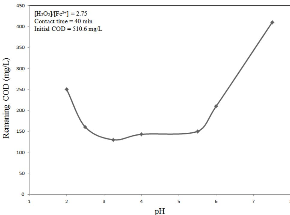
**Figure 1: Effect of pH on the removal of chemical oxygen demand (COD) by Fenton's treatment for the biologically treated HD-SBR landfill leachate**
