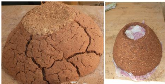
Figure 3: Extent of crack in the bodies made by micro (left) and macro (right) granularity
