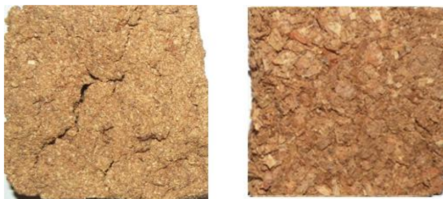
Figure 2: Difference between cracks in micro- (left) and macro- (right) granularity bodies
