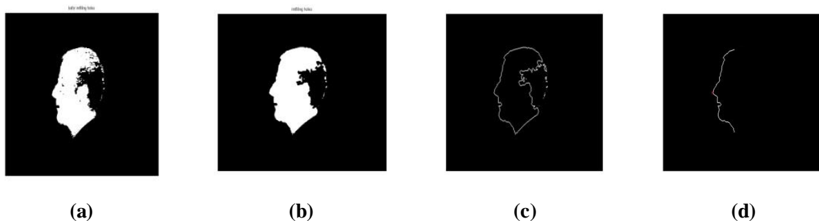
Figure 5: The probability image: (a) Raw grayscale mode, (b) after applying morphological operations(c) Edge detection for binary image of pervious stage and (d) Profile extracted applying boundary of rectangular region for profile face
