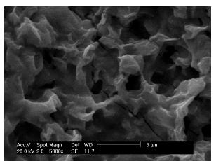
Figure 2: Scanning electron microscopy of cadmium sulfide on glass thin layers for 25 min time deposition
