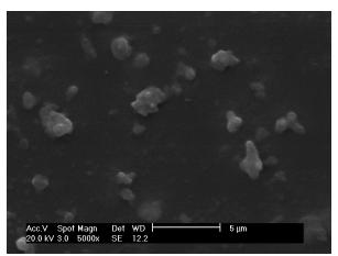
Figure 3: Scanning electron microscopy of cadmium sulfide on glass thin layers for 45 min time deposition
