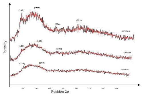
Figure 4: XRD pattern of CdS films grown at three different time deposition.
