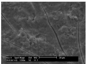
Figure 1: Scanning electron microscopy of cadmium sulfide on glass thin layers for 15 min time deposition
