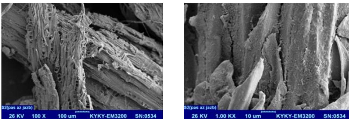
Figure 10: SEM images after adsorption of metal by Eucalyptus sawdust with 100X and 1KX magnifications
