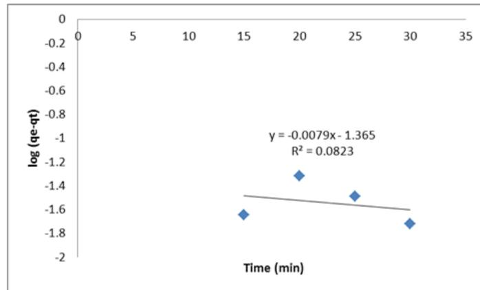
**Figure 7: First-degree adsorption kinetic model**
