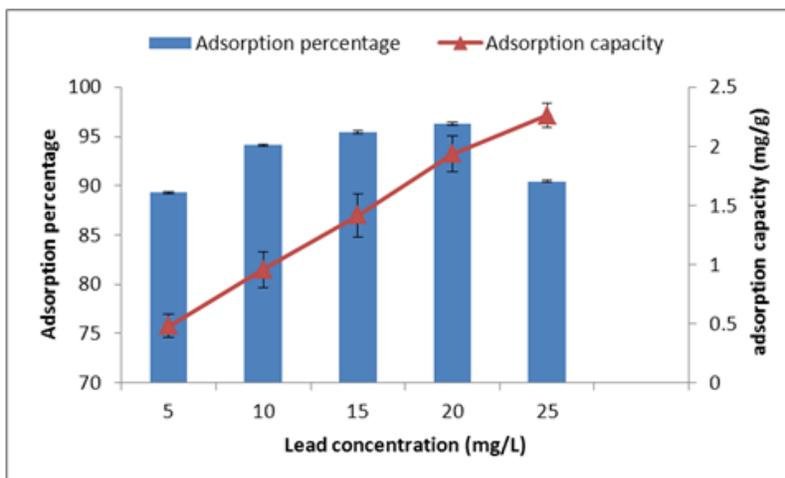
**Figure 4: Effect of the quantity of different initial concentration on the capacity and percentage of lead (pH=7, Adsorbent quantity =10 g/L, Contact time=30 min)**
