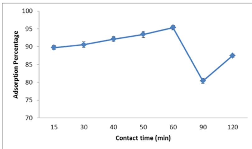
**Figure 3: Effect of different contact times on the adsorption percentage of lead (pH=7, Adsorbent quantity =10 g/L, Initial concentration of lead=10 mg/L)**
