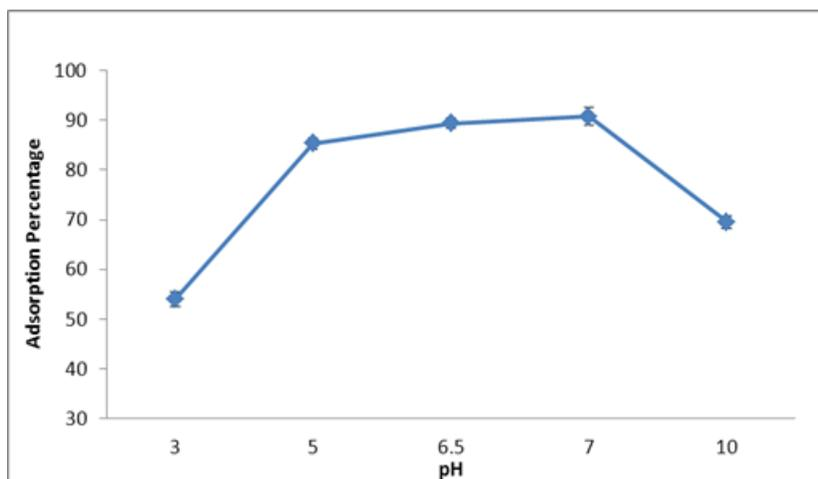
Figure 1: Effect of various pH on the adsorption percentage of lead (Adsorbent quantity =10 g/L, Contact time=30 min, Initial concentration of lead=10 mg/L)
