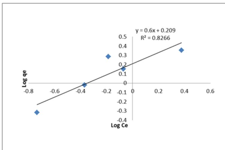
**Figure 6: Freundlich isotherm model for lead adsorption**
