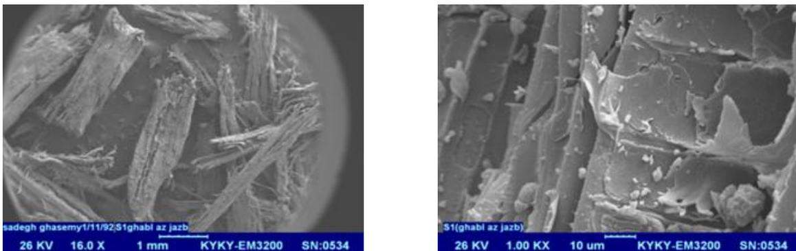
Figure 9: SEM images before adsorption of metal by Eucalyptus sawdust with 16X and 1KX magnifications
