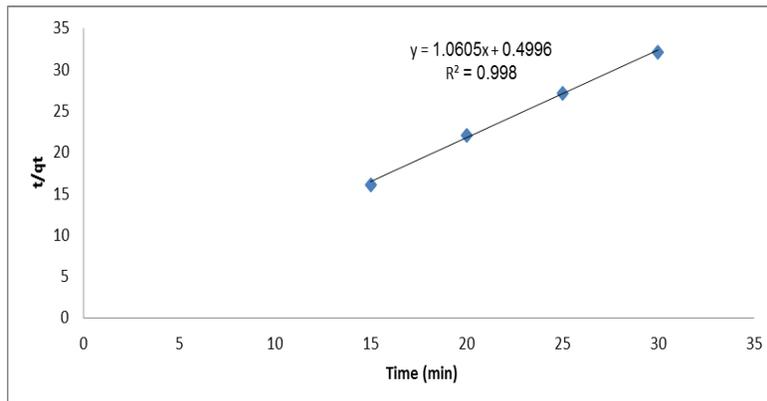
**Figure 8: Second-degree adsorption kinetic model**
