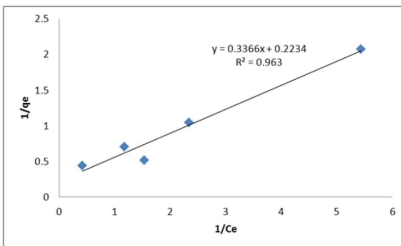
**Figure 5: Langmuir isotherm model for lead adsorption**
