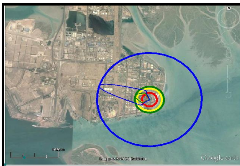
Map 3: NO 2 dispersion from Flue 3 (with abnormal percent) of VCM unit in Bandar Imam Khomeini Petrochemical Complex in winter
