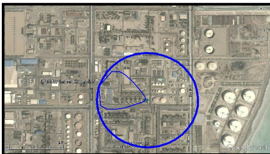
Map 1: Dispersion of NO 2 from Flue 3 of VCM unit in Bandar Imam Khomeini Petrochemical Complex in winter
