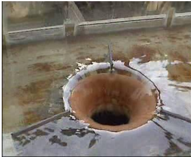
Figure 1: A view of the physical model of shaft spillway with vortex breaker structure in laboratory
