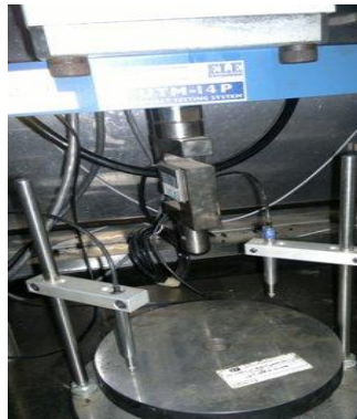
Figure 5: Scheme of loading shaft and measurement sensors of UTM deformation
