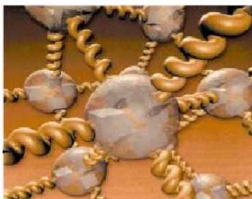
Figure 3: Schematic design of combination of SBS molecules with bitumen, polymer volume increases 9 times after exposure to bitumen (Morgan and Mulder, 1995)
