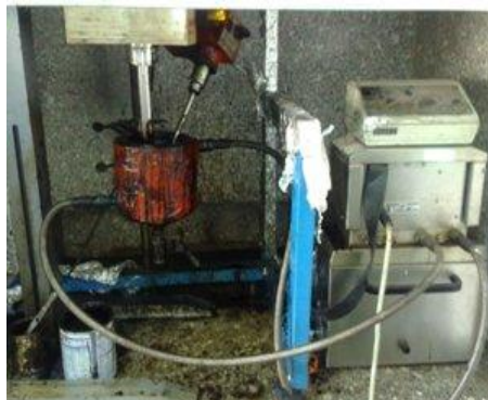
Figure 4: Mixer having the shear and rotation shafts for production of polymer bitumen
