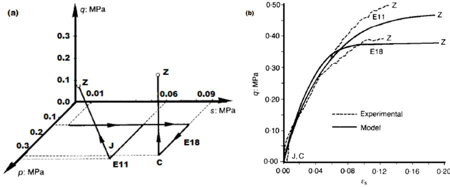
**Figure 2: Shear tests on partially saturated compacted kaolin: (a) stress paths; (b) comparison of measured and predicted shear stress- strain relationships (after Alonso *et al.*, 1990)**
