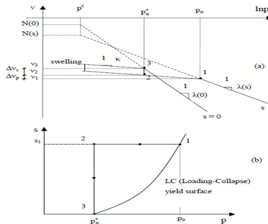
**Figure 1: (a) Assumed isotropic compression lines, and (b) LC yield surface (after Alonso *et al.*, 1990)**
