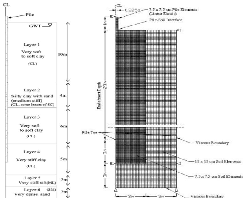
**Figure 5: (a) The axisymmetric pile-soil model for pile driving simulation. (b) Geometry, mesh and boundaries of the axisymmetric pile-soil numerical models- the Finite Difference Method (FDM) (Fakharian *et al.*, 2014)**
