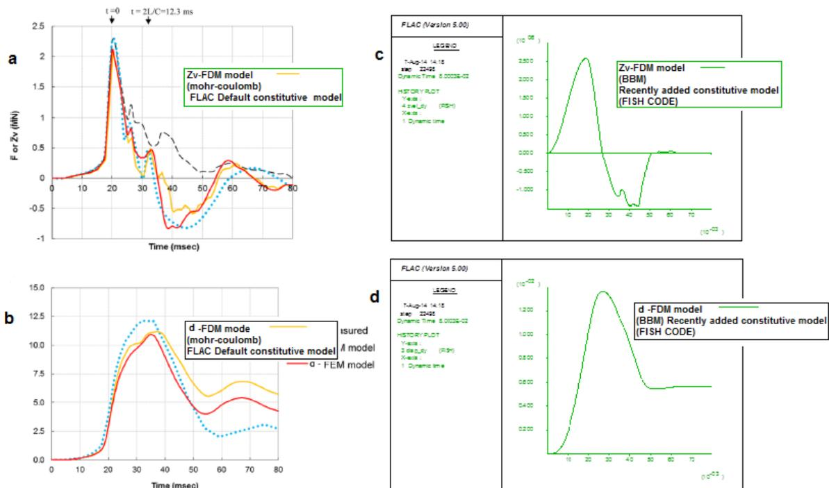
**Figure 7: Comparing the results of the response of pile driving finite difference model based on BBM constitutive model with pile driving finite difference model based on M-C constitutive model**
