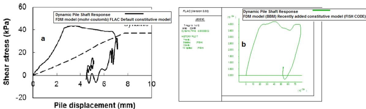
**Figure 8: Comparing the results of dynamic load carrying capacity of pile driving finite difference model based on BBM constitutive model with pile driving finite differenced model based on M-C constitutive model**
